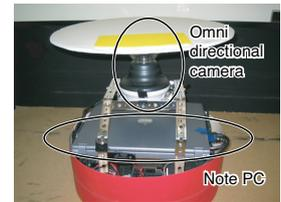
(c) Objective robot with an omnidirectional camera
