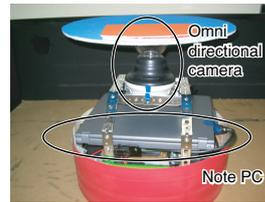
(b) Hunter robot with an omnidirectional camera
