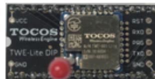
Fig.2 Wireless communication device: TWE-Lite DIP
