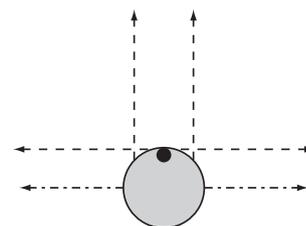
Fig. 3 Ray of the distance sensors (dash line) and the target detection sensors (dot-dash line)
